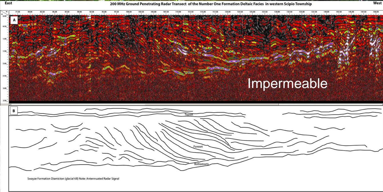
Image A is processed radar record; Image B is interpreted line drawing
